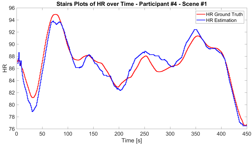
Figure 3.15: Example of stairs plot: it represents the HR GT and estimations over time.
