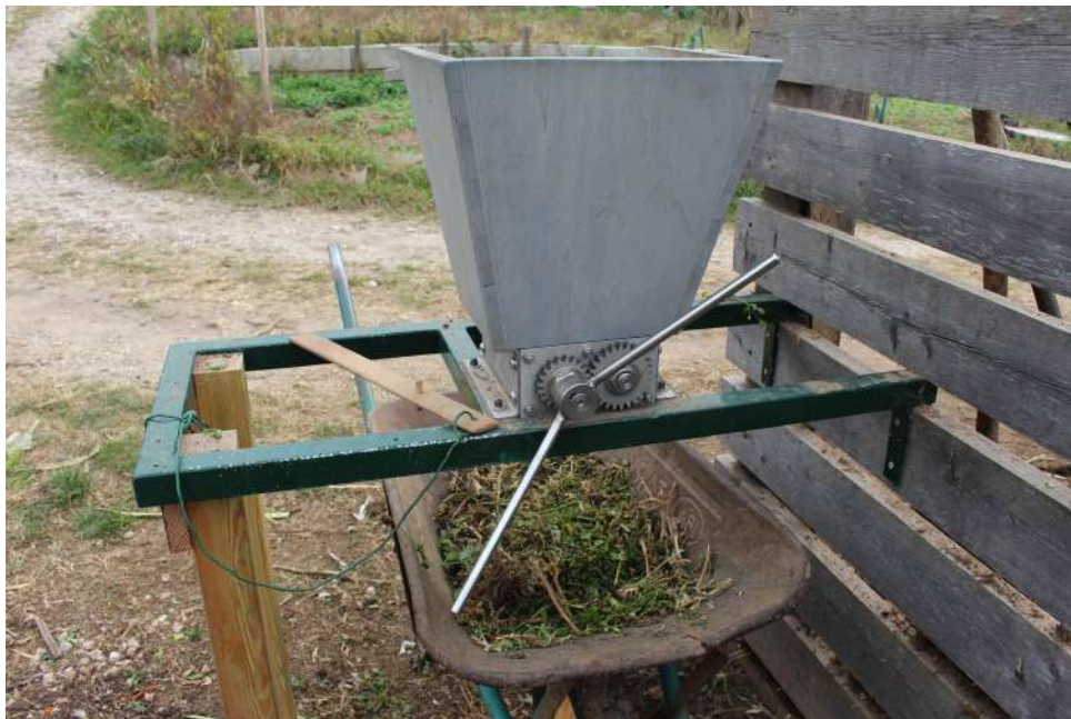
Figure 7.21: The crank-powered shredder.
