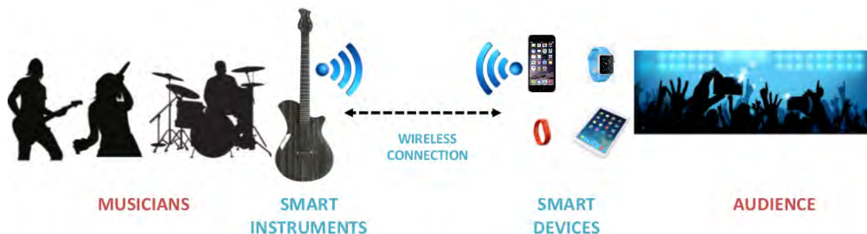
Figure 1. A schematic representation of the bidirectional wireless connectivity between Smart Instruments and smart devices enabling new forms of interaction between performers and audience.
