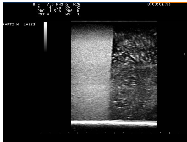
Figure 2: B-mode image recorded at MI of 0.4. Tissue mimicking phantom (TMP) and C2 type nanodroplets (NDs) are shown.
