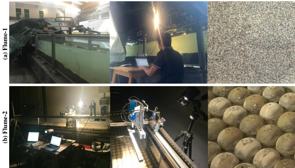
322 Fig. 1. Spectroscopic experiments in a range of water depths on (a) flume-1 with a sand bed and (b) flume-2 with a 323 gravel bed composed of semi-natural material.
