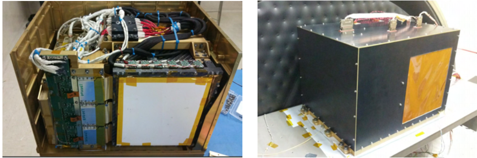
Figure 6: Picture of the HEPD flight model (FM): assembly (left) and at the thermal-vacuum acceptance test (right).
